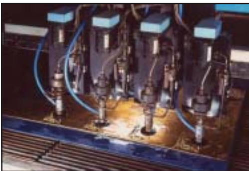
Abrasive waterjet cutting .25" brass four parts at a time
