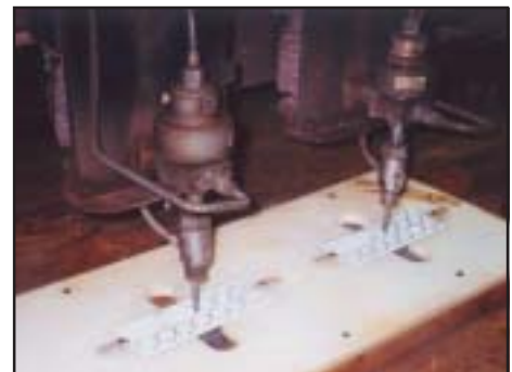
Abrasive waterjet cutting .030" ceramic coated .125" steel
