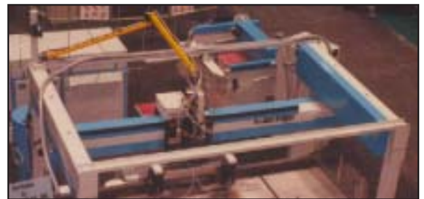
Scissor style UHP plumbing (yellow assembly)
